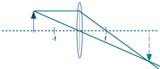
With the bi-convex lens a larger, real image is formed when the object is placed  $>f$  away from the lens. This kind of image can be seen on a screen
