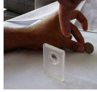
In Part 4), students work with the bi-convex lens to find out that when the object is placed before the focal point ( $< 30$  mm away from the lens) then no sharp image is seen on the screen. The rays diverge as shown in the ray diagram below and a virtual image is formed.
